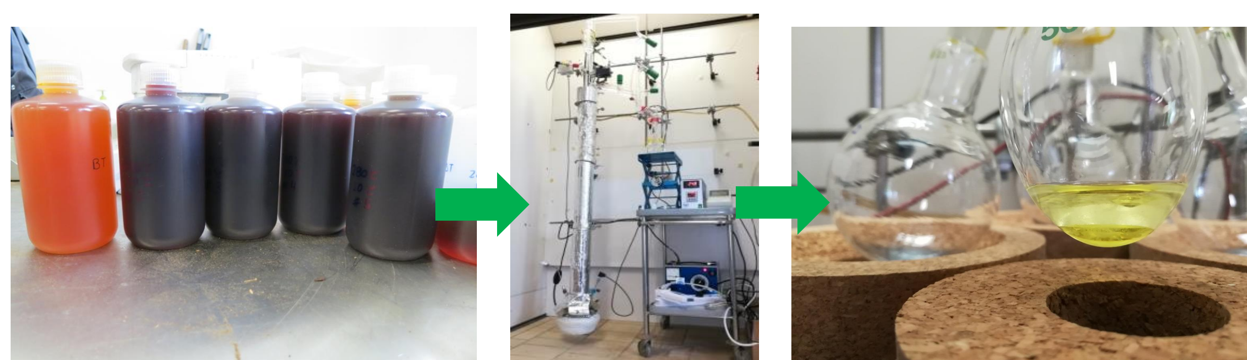
Figure 1. Batch rectification column with initial condensate and obtained furfural fraction.
